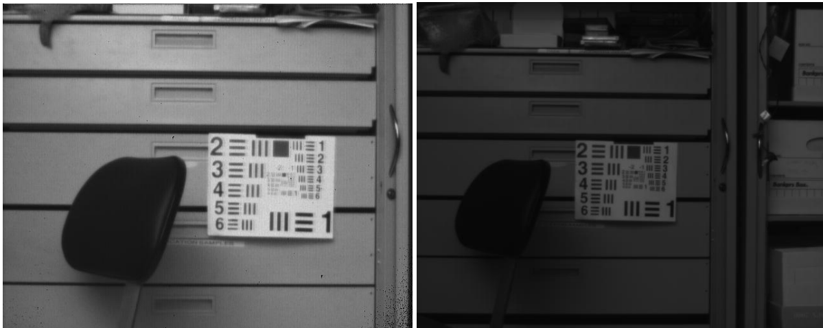
Figure 6. Images from the camera designed for PCAR (left) and 640SDX camera (right) in low light level laboratory environment with Tungsten lamp illumination only.
