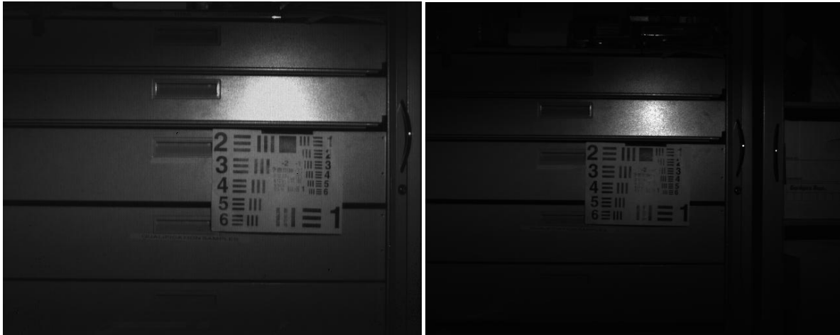
Figure 7. Images from the camera designed for PCAR (left) and 640SDX camera (right) in low light level laboratory environment with 1550 nm LED illumination only.
