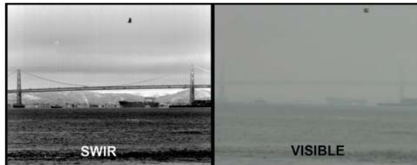
Figure 4. Comparative SWIR (left) and visible (right) images of a San Francisco Bay Bridge scene with typical morning fog
