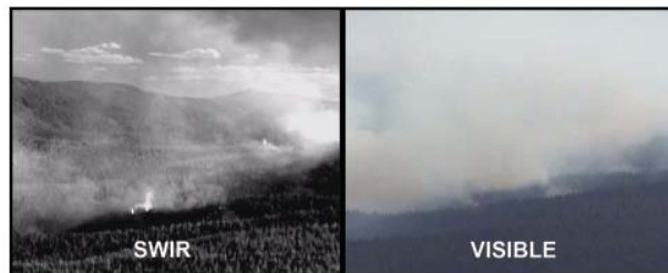
Figure 5. Comparative SWIR (left) and visible (right) images of an Oregon forest fire scene (images courtesy of Cloud Cap Technologies)
