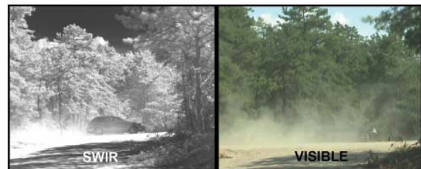
Figure 3. Comparative SWIR (left) and visible (right) images taken in the dusty Pine Barrens of southern New Jersey
