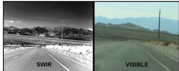
Figure 2. Comparative SWIR (left) and visible (right) images of haze taken on the approach to Death Valley, CA
