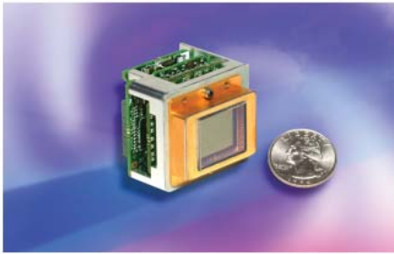
Figure 1. Sensors Unlimited SU640KTSX InGaAs NIR/SWIR Camera (OEM version). The 640 x 512 pixel format camera features a 25 \mu\text{m} pixel pitch focal-plane array responsive from 0.7 - 1.7 microns and gathers full-sized images at 30 fps.
