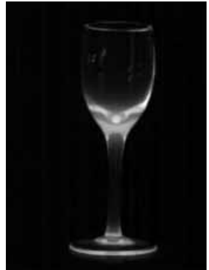
Figure 3. A thermal camera could see only the top surface of this wine glass, still in the “hot end” stage of production. SWIR provides a false-color temperature profile on all surfaces. (Photo by Martin Ettenberg.)
