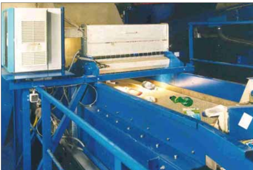
Figure 4. Linescan SWIR imagers are at work classifying polymers for sortation on a recycling line in Europe. Some types of plastic can be given a new life as other products, including coats and outdoor furniture.
