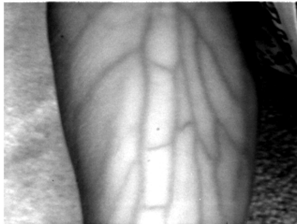
Figure 1: Forearm viewed in the short-wave IR with an InGaAs (indium gallium arsenide) camera
