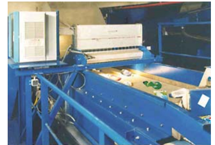
SWIR cameras classify polymers for sorting on recycling line in Europe.
