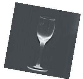
The false-color temperature profile of a wine glass taken with SWIR lets inspectors see all surfaces, not just the front or surface facing the camera.
