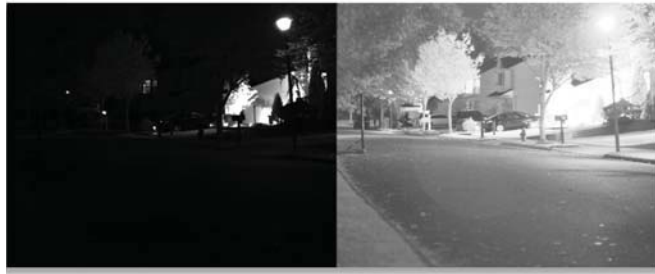
Figure 2: Nighttime SWIR imaging in an urban environment. Unenhanced, raw data image (left); enhanced data image (right).
