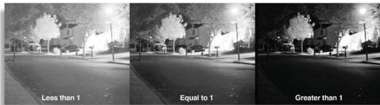
Figure 4: Effects of the POWER function on SWIR urban night imagery. From left to right, a POWER value less than 1, equal to 1, and greater than 1.
