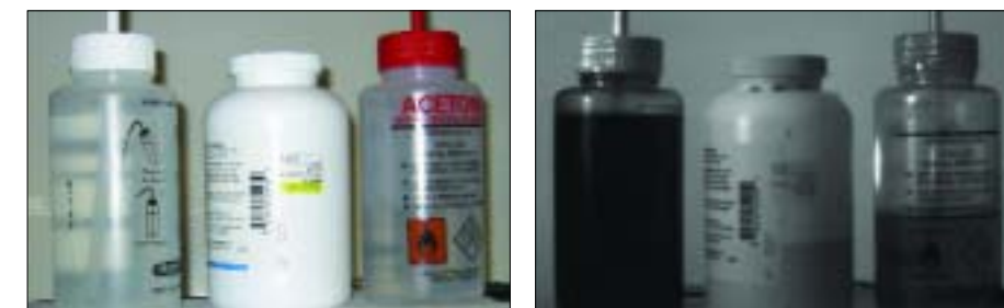
Fig. 2. Short-wave imaging (right), unlike visible imaging (left), can be used to see through plastic and determine liquid levels inside opaque containers.
