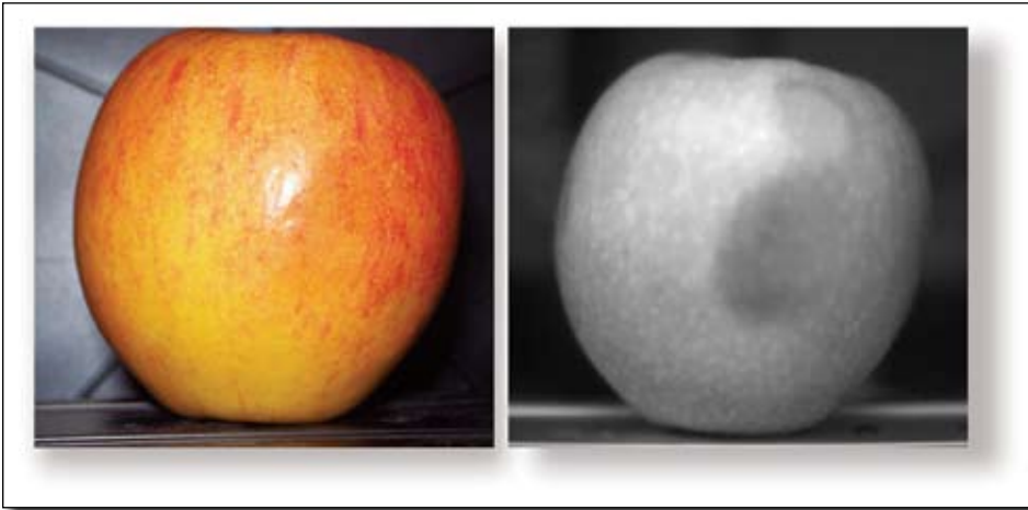
Fig. 2 – Visible apple image (left) and SWIR apple image (right) clearly shows bruising
