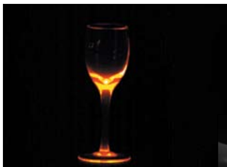
Figure 3: A hot wine glass in false color, imaged using a Sensors Unlimited, Inc. 320x240 InGaAs MiniCamera. The signal levels can be calibrated to temperature; in this case, the hottest part of the glass is 330°C (above). The second image shows the same glass with a business card behind it, demonstrating that glass is completely transparent in this wavelength band (right).
