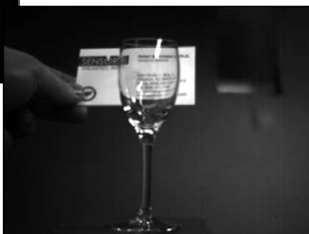
Figure 3: A hot wine glass in false color, imaged using a Sensors Unlimited, Inc. 320x240 InGaAs MiniCamera. The signal levels can be calibrated to temperature; in this case, the hottest part of the glass is 330°C (above). The second image shows the same glass with a business card behind it, demonstrating that glass is completely transparent in this wavelength band (right).
