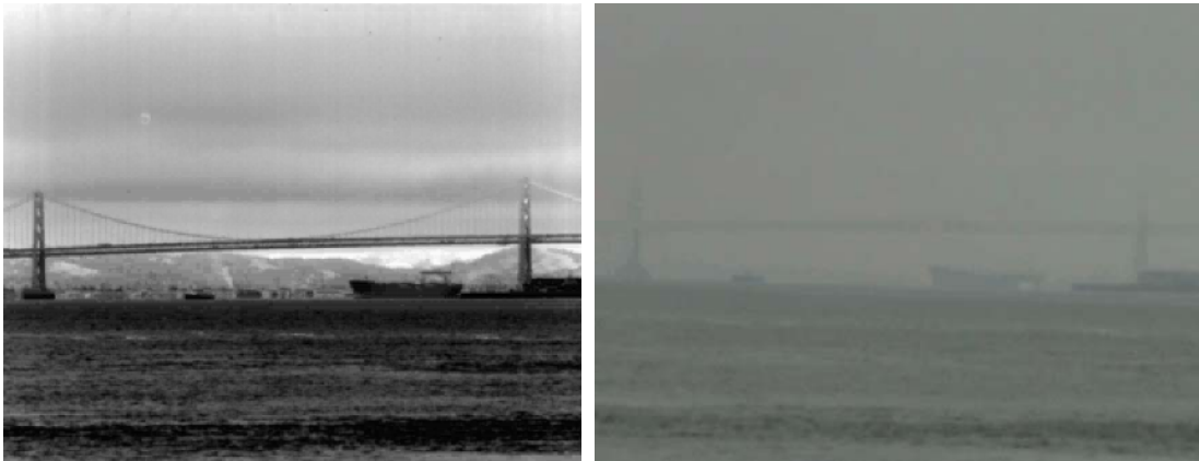
Figure 2: Daytime movies in San Francisco Bay. Click on each and note the small boat crossing in front of the large freighter, a white box in the visible, clearly seen in the SWIR.
