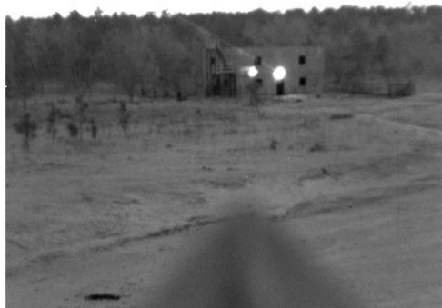
Image of 0.8 and 1.5 \mu\text{m} lasers taken with Goodrich's 320KTX NIR/SWIR InGaAs camera.
